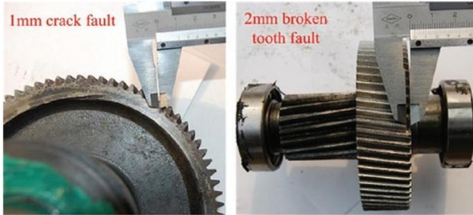
Fig. 5. Location of compound fault in gears
